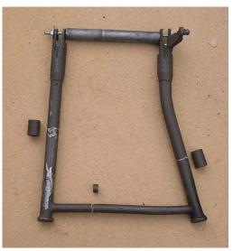
Cut the right leg and the horizontal bar and push the stub in the other half of the left leg. You can now scribe the length of pipe to be removed from the right leg and the horizontal bar,
