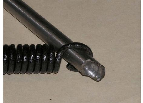
Then the 50 penny method: find a stack of pennies (or suitable washers), bend the spring and insert a penny on one side. Bend in the opposite direction, and insert another penny, and so on. In theory this will stretch the spring enough to hook it over the mushroom. But no luck, I could not even insert 10 pennies (in my case: Euro 2 cent pieces).
