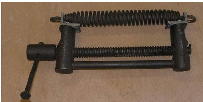
For the rest, look at the pictures; never mind the workmanship, I was in a hurry and it works which is the most important thing. The two small forks grip the spring ends, then you turn the screw and the spring is stretched and stretched safely until it slips over the mushrooms, and Bob's your uncle as the 'murricans say. And of course removing the spring also becomes easy.
